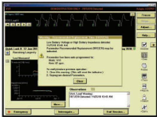
Example 1 – Programmer Software Detects Measurement Lock-up ERI
